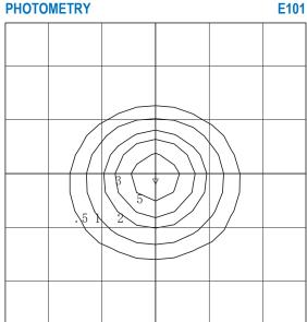
Horizontal Footcandles Scale: 1 Inch = 8 Ft. Light Loss Factor = 1.00 Lumens Per Lamp = 1749.8 Total Lamp Lumens = 1749.8 Mounting Height = 10.00 Ft Maximum Calculated Value = 7.18 Fc Arrangement: Single
