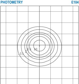
Horizontal Footcandles Scale: 1 Inch = 15 Ft. Light Loss Factor = 1.00 Lumens Per Lamp = N.A. (absolute photometry) Luminaire Lumens = 9073 Mounting Height = 15.00 Ft Maximum Calculated Value = 16.26 Fc Arrangement: Single
