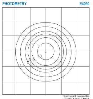
Scale: 1 Inch = 12 Ft. Light Loss Factor = 1.00 Lumens Per Lamp = N.A. (absolute photometry) Luminaire Lumens = 9838 Mounting Height = 15.00 Ft Maximum Calculated Value = 16.85 Fc Arrangement: Single
